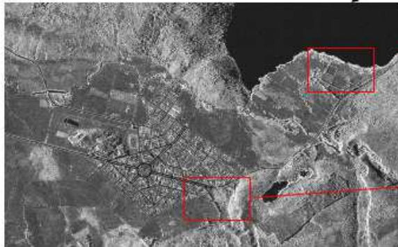
Fig. 3: AFrost filter applied to Cosmos image (HH) showing a partial view. Blocs, rows, water and high vegetation is recognized
