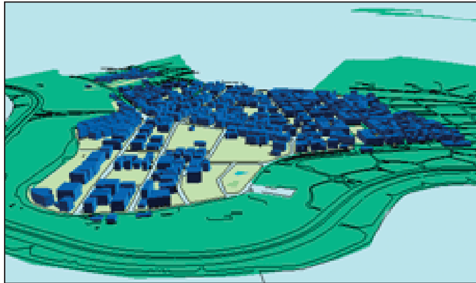
ArcView 3D Analyst was used to extrude buildings for a three-dimensional view of the pilot study area.
