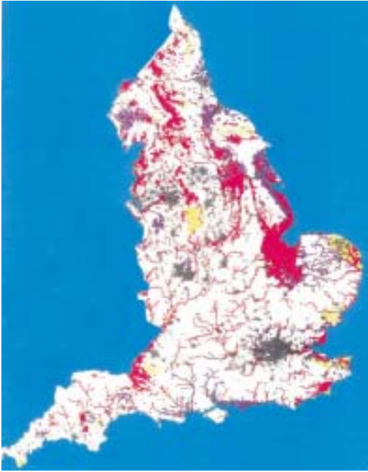
Figure 2A4. Compressibility of the ground in England (after Wimpey Environmental, 1995)
