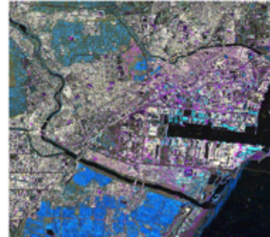
Sendai, Japan, after the tsunami on March 11, 2011, based on TerraSAR-X radar images. Inundated areas appear in blue, debris in magenta and affected infrastructure in cyan blue. (Image DLR-DFD, ZKI)
