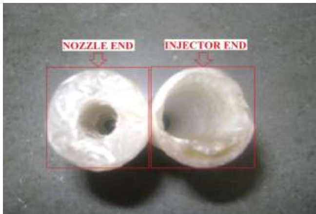
Figure 3.2 regression rate behaviours of injector and nozzle end
