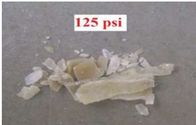
Figure 3.1 sliver at 125psi injection pressure
