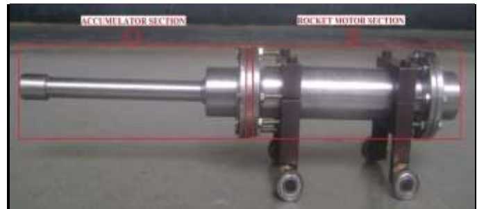
Figure 2.1, Hybrid motor assembly without VG
