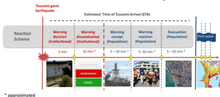
Reaction scheme of a people-centred tsunami early warning system developed in the context of GITEWS (Image: DLR)
