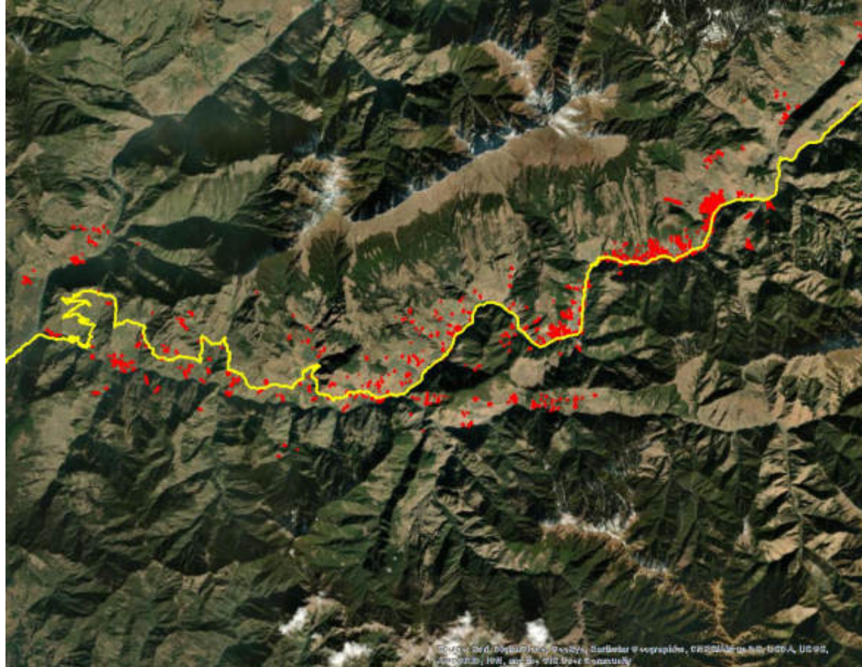
Landslides between Manma and Jumla section directly impacting the Karnali highway – mapped using recent Planet imagery and SALaD-CD
