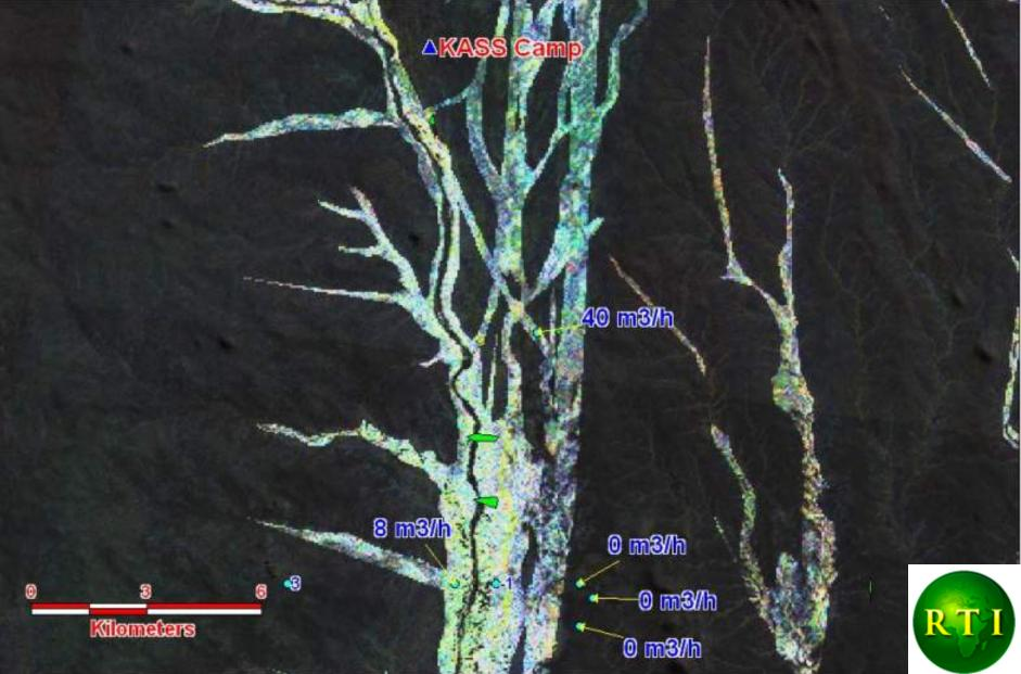
WATEX© application in Chad to identify conductive fractures and drill wells for the refugees of Iridimi Camp
